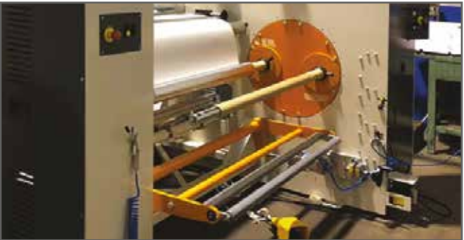
In-feed and Out-feed Turret systems
